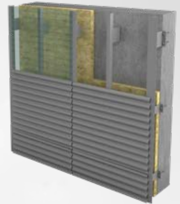
ALWI-S with horizontally installed aluminium corrugated profile panels
